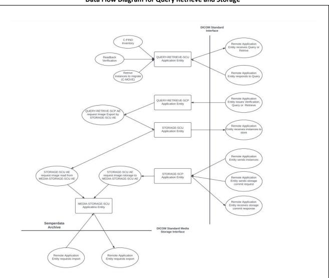
Figure 3.1-1 Data Flow Diagram for Query Retrieve and Storage
