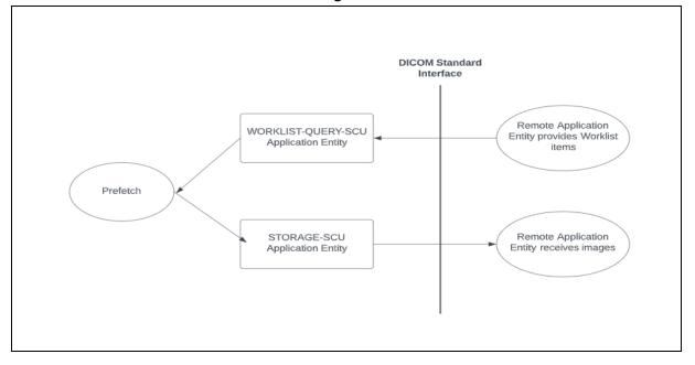
Figure 3.1-4 Data Flow Diagram for Query-Retrieve *(see first data flow diagram)*
